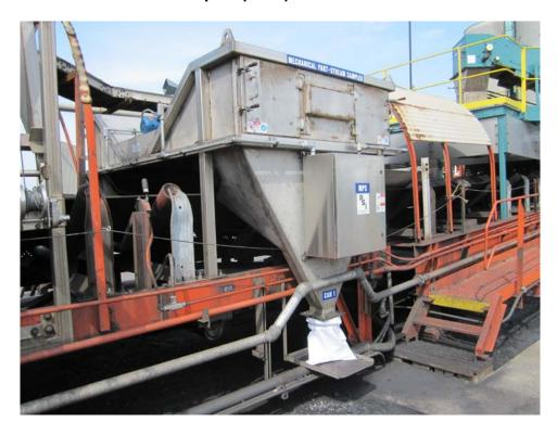
The Mechanical Part-stream Sampler (MPS) is primarily an alternate mechanized sampling device that can be placed into service in the event the AS is inoperable. Having this back-up sampling device available eliminates the need for personnel to manual sample off the conveyor, and thus avoids potential safety hazards associated with that sampling method. The MPS can also be used in tandem with the AS to collect extra uncrushed sample material for a size analysis or other special test.
