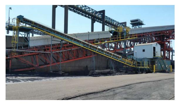
The system's key components are listed below and operate to meet or exceed ASTM standards when accepting a product of 75 mm  $\times$  0 (3 in.  $\times$  0) or less. The sampling system can be tailored to operate at multiple belt speeds and cutter frequencies to accommodate special sample requests down to consignments of 1,000 tons.
