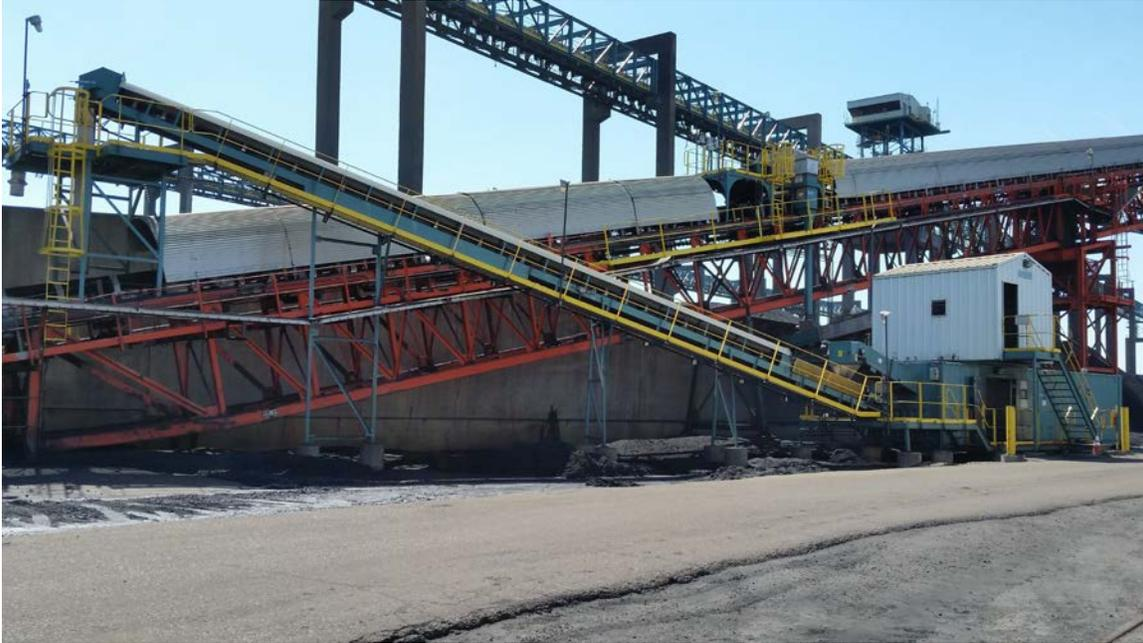
The system's key components are listed below and operate to meet or exceed ASTM standards when accepting a product of 75 mm x 0 (3 in. x 0) or less. The sampling system can be tailored to operate at multiple belt speeds and cutter frequencies to accommodate special sample requests down to consignments of 1,000 tons.
