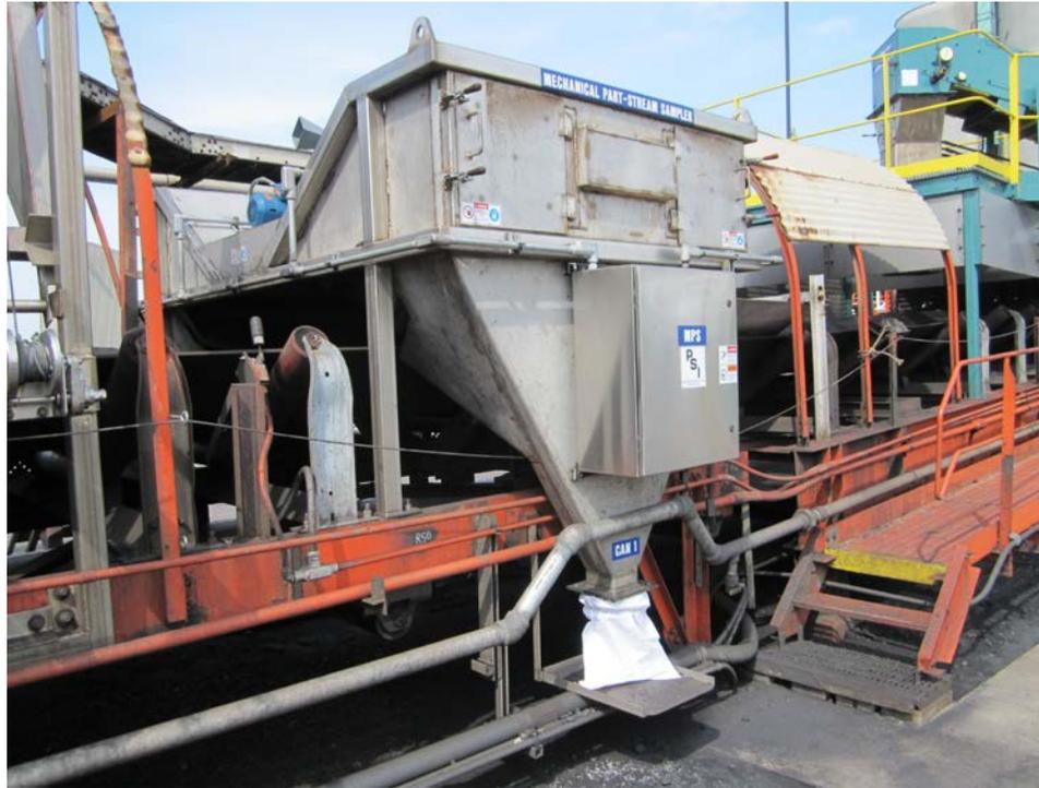
The Mechanical Part-stream Sampler (MPS) is primarily an alternate mechanized sampling device that can be placed into service in the event the AS is inoperable. Having this back-up sampling device available eliminates the need for personnel to manual sample off the conveyor, and thus avoids potential safety hazards associated with that sampling method. The MPS can also be used in tandem with the AS to collect extra uncrushed sample material for a size analysis or other special test.
