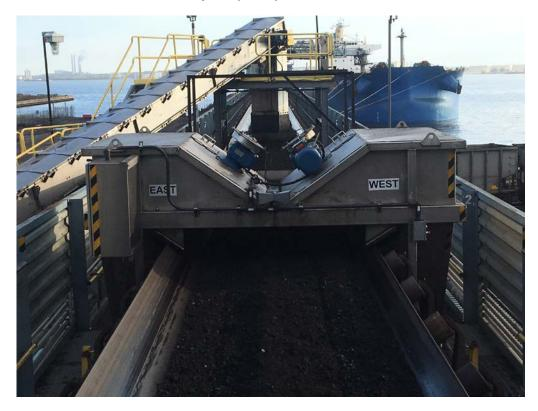
The Mechanical Part-stream Sampler (MPS) is primarily an alternate mechanized sampling device that can be placed into service in the event the AS is inoperable. Having this back-up sampling device available eliminates the need for personnel to manual sample off the conveyor, and therefore avoids potential safety hazards associated with that sampling method. The MPS can also be used in tandem with the AS to collect extra uncrushed sample material for a size analysis or other special test.
