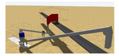
**Primary Sampler** - This cross-belt component (red) operates at a minimum 1.5 times the speed of the C-2 conveyor (black) where it extracts a 70.7 kg (155.8 lb.) increment every 35 seconds. The cutter opening is 228 mm (9.1 in.) in width. A plugged-chute indicator and a vibrator are installed on the transfer chute between the Sampler and the Primary Feeder Conveyor to facilitate material flow. Sample material is gravity-fed to the Primary Feeder Conveyor.
