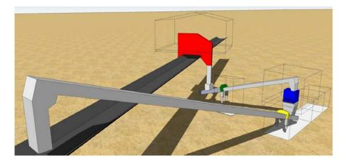
**Primary Sampler** - This cross-belt component (red) operates at a minimum 1.5 times the speed of the C-6 conveyor (black) as it extracts a 71.8 kg (158 lb.) increment every 29 seconds. The cutter opening is 225 mm (9 in.) in width. Each primary increment is gravity-fed to the Primary Feeder Conveyor. A plugged-chute indicator and a vibrator are installed on the transfer chute between the Sampler and the Primary Feeder Conveyor to facilitate the flow of material.
