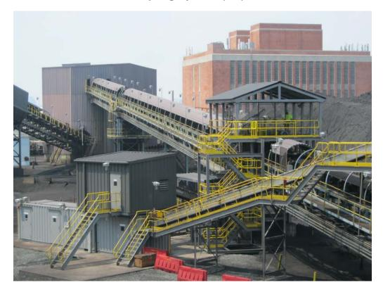
The system's key components are listed below and operate to meet or exceed ASTM standards when accepting a product of 75 mm  $\times$  0 (3 in.  $\times$  0) or less. The system can be set to operate at multiple belt speeds and cutter frequencies to accommodate special sample requests for consignments down to 5,000 tons.
