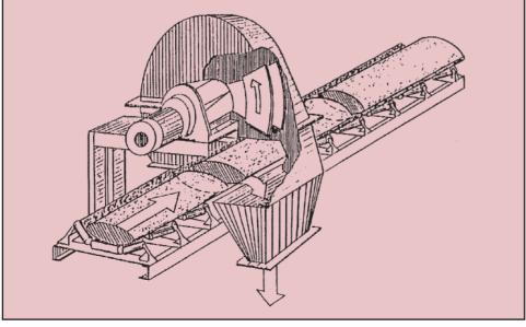
Figure 4. Cross belt or sweep arm sampler.
