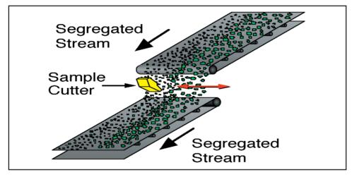
Figure 3. Sample collection at a transfer point between two conveyor belts.
