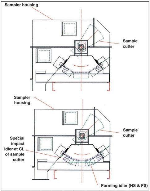
Figure 5. Comparison of sampling stations; above, the unmodified station and below a sampling station fitted with special impact idlers to generate a perfect belt contour.
