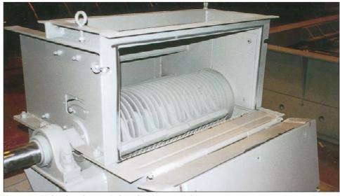
Figure 7. Mclanahan Corp. crusher showing ease of access.
