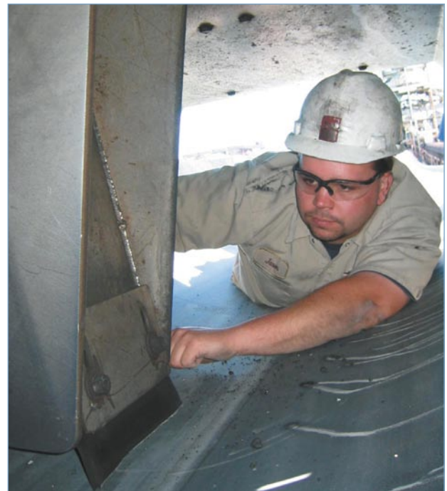
Figure 4. Adjusting the primary sampler belt wiper.
