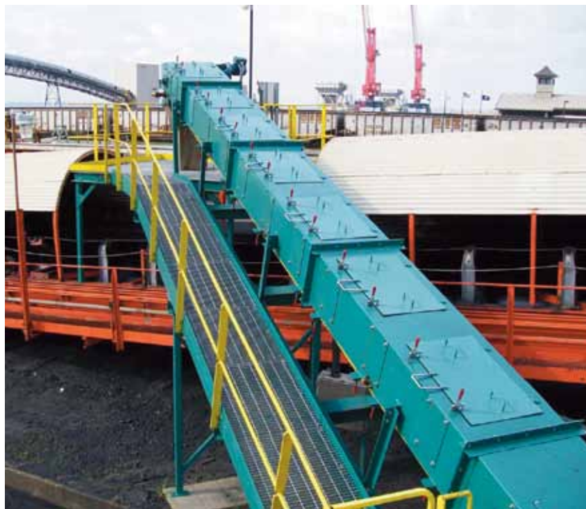
Figure 6. Conveyor with excellent maintenance access.
