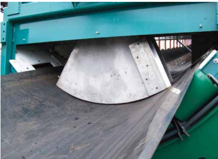
Figure 1. Contour arc with impact and shaping idlers.
