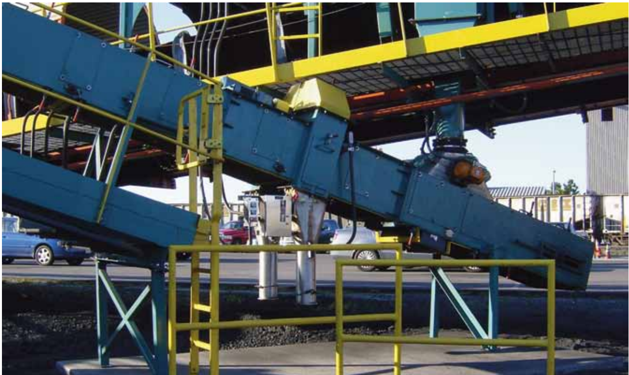
Figure 4. Mechanical sampler for sizing.
