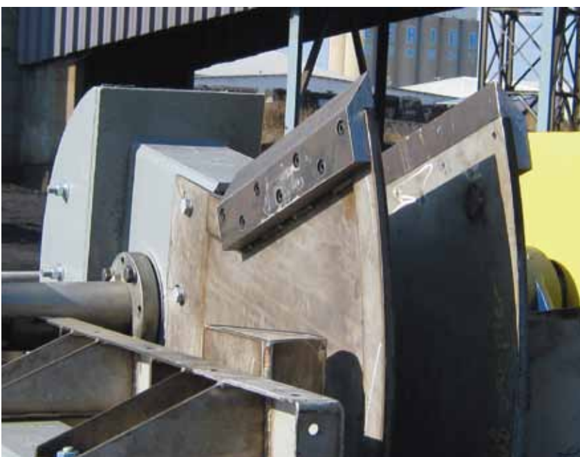
Figure 2. Bevelled and replaceable cutter lips.
